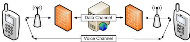
Figure 1. Mobile to mobile connections illustrating voice and data channels, the latter restricted by firewalls.
